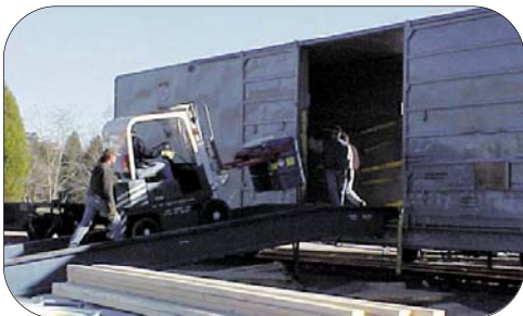
MHF-LS boxcar with drum securement and spill containment system being loaded for shipment.
