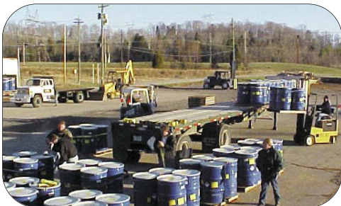
Drums of mixed hazardous waste being off loaded from truck and staged for loading in MHF-LS boxcar.
