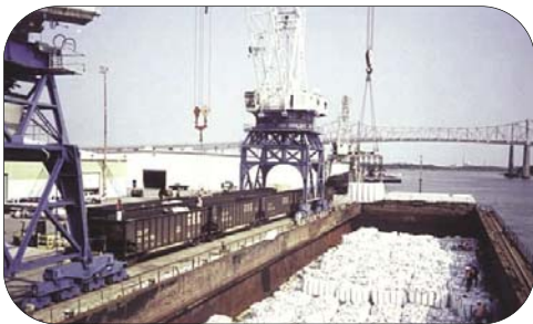
Lift Liner™ bulk bags being transloaded from barge to rail.
