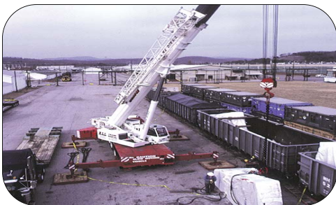
Overweight cargo being off loaded from rail to truck for final delivery.
