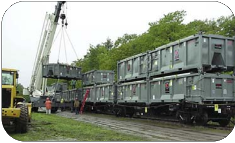
Intermodal containers being loaded onto ABC flatcars at a remote site.
