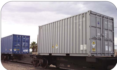
MHF-LS flatcars containing sealand containers for rail-to-truck transfer to disposal site.
